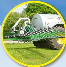
Integrated "anti-drip" lifting device (TWIST system)
